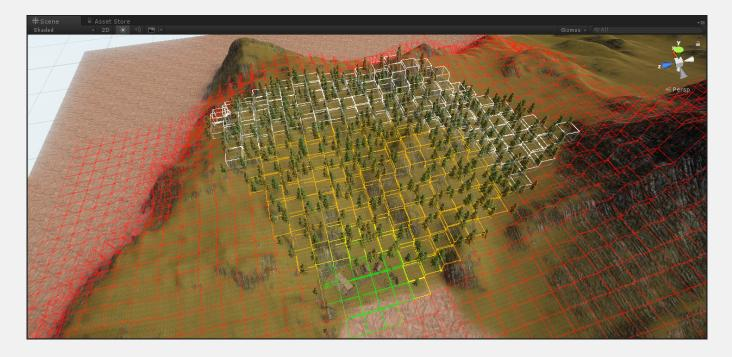
In order to handle fast culling and rendering of vegetation, VegetationSystem will split the terrain into cells. These are then culled using the CullingGroups API. Enable this option to see the current visible cells in sceneview. Cells are color coded based on visible LOD, Green, Yellow and Orange for vegetation distance and white for additional tree range.
